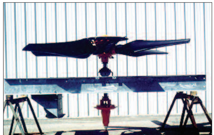
Inverted Actuator-Variable-Pitch Fan Fig. 15
