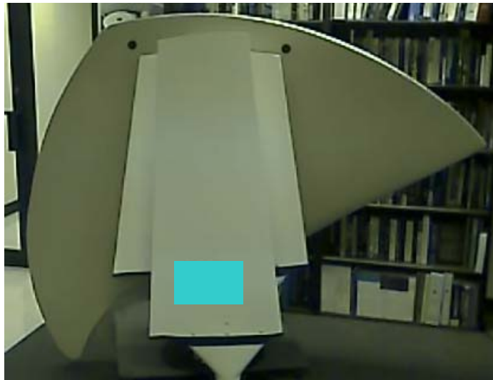
Figure 7. Size comparison of standard noise (foreground), very low noise (middle) and ultra low noise (back) fan blades
