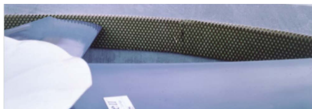
▲ Figure 8. A tip seal retrofit can correct excessive tip clearance and improve fan performance.
