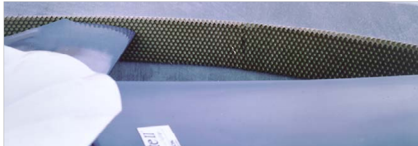
Figure 6. Typical tip seal retrofit
