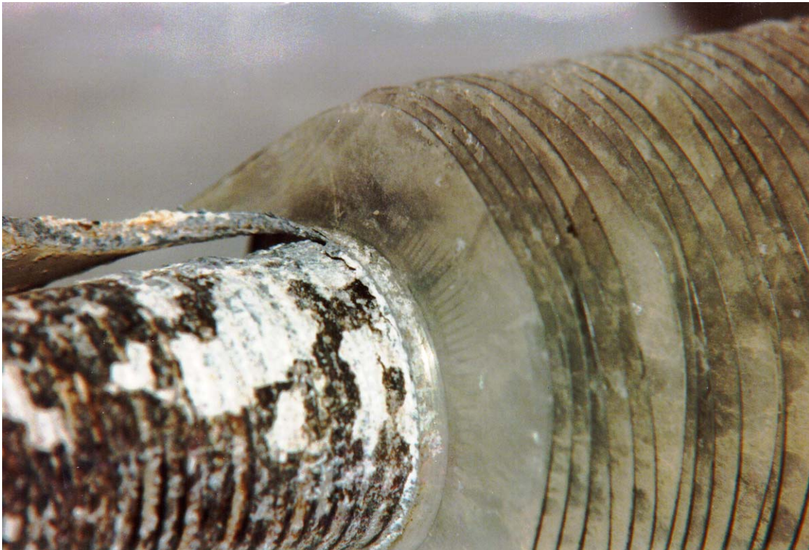
Figure 11. Effect of water spray on L-Base fins
