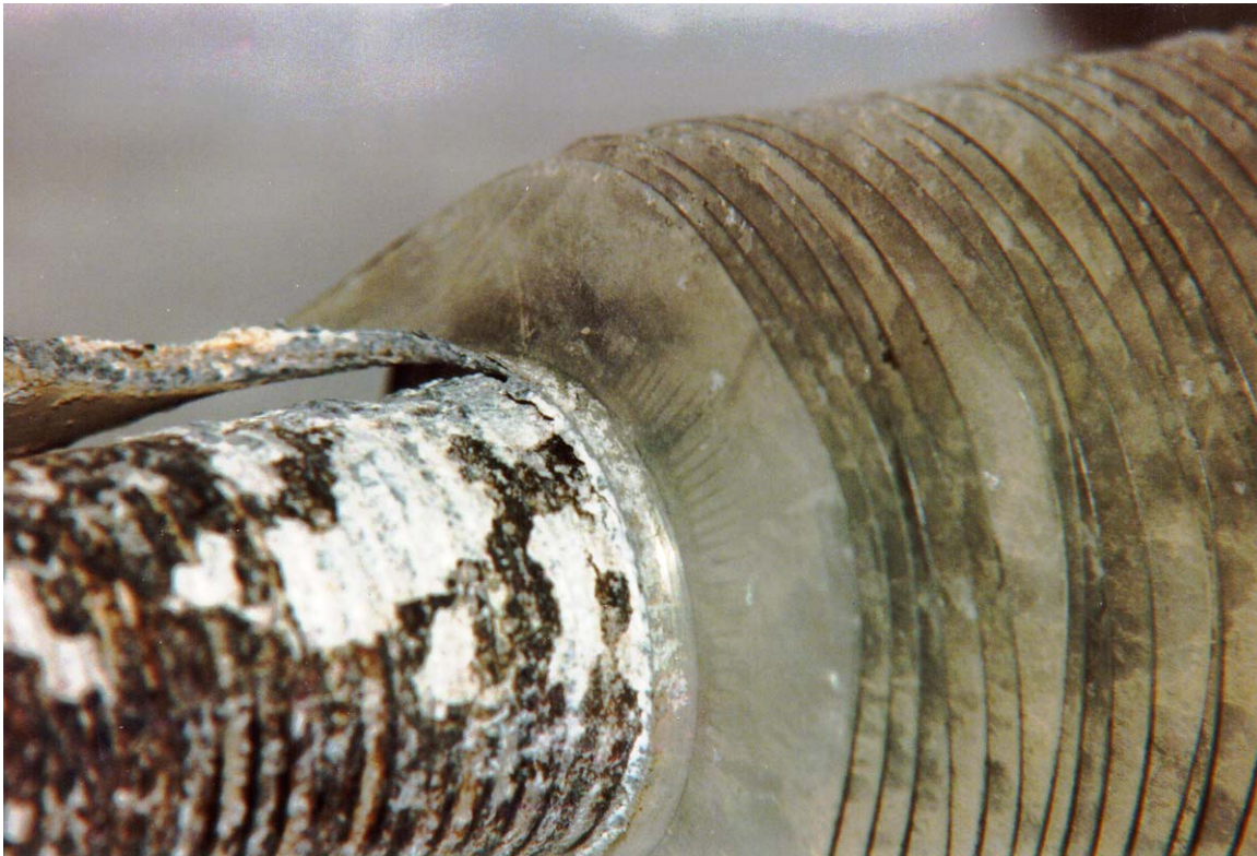
Figure 11. Effect of water spray on L-Base fins
