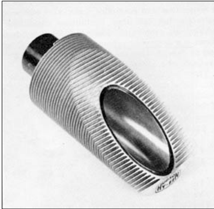
Figure 9 Extended heat-exchanger surface consists of extruded aluminum fins over a carbon-steel tube
